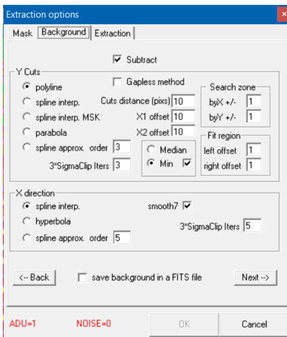
Figure 63 The second panel for setting extraction parameters. Settings for taking into account scattered light.
