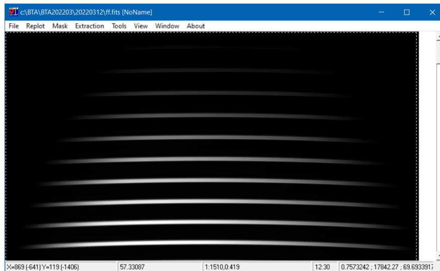
Figure 5 Image of a flat field in the black and white mode.
